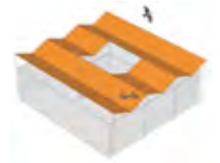
Fig. 19 ROOF – collection at four points (1 interior, 3 exterior).
